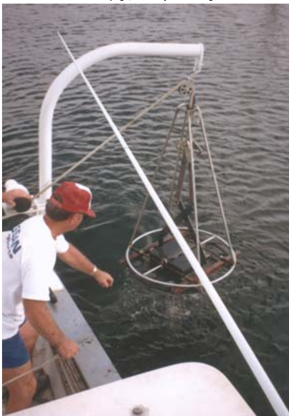
Sampling using a Ted-Young modified VanVeen. Large grab samplers such as these require winches and sufficient boat size for efficient operation.
