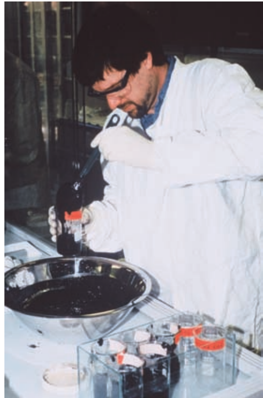
Subsampling sediment for toxicity testing
